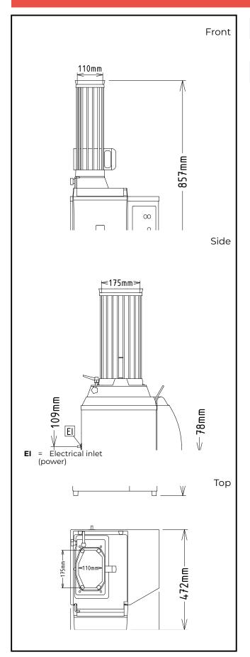
Electric Supply voltage: 220-240 V/1N ph/50 Hz **Total Watts:** 0.37 kW Key Information: External dimensions, Width: 472 mm External dimensions, Depth: 418 mm External dimensions, Height: 857 mm Net weight (kg): ISO 9001; ISO 14001
